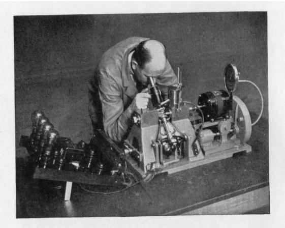
MAKING SURE sometimes tests the ingenuity of even Nuffield engineers. In order to use this machine, one of three of the kind in existence, it was necessary to evolve a special technique. Study with the aid of this apparatus yields valuable information about the film of oil necessary to give adequate protection to metal surfaces under conditions varying from arctic cold to tropical heat.
