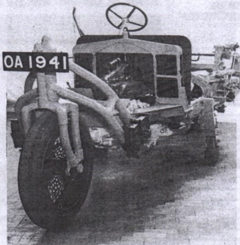
Naked Gyrocar shows leaf springs, outrigger wheels and immense chassis.
