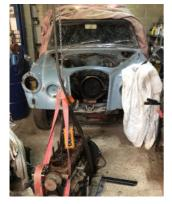
A car unlikely to make it on to the road in 2024 is this 1966 6/110 Mk II automatic which belongs to Martin Cooper and his son Jacob, from Kent. It's been stored for more than 30 years, and the pair have just embarked on its restoration. Martin laid the car up after partially seizing the engine "being the naïve youth I was." They have rebored the engine and fitted new pistons, and other mechanical work is well under way.
